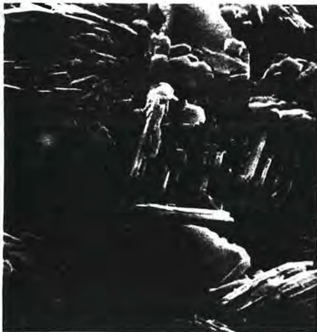
Fig. 3.11 Electron photomicrograph of well-crystallized kaolinite from St. Austell, Cornwall, England. Picture width is 17\ \mu\text{m} (Tovey, 1971).
